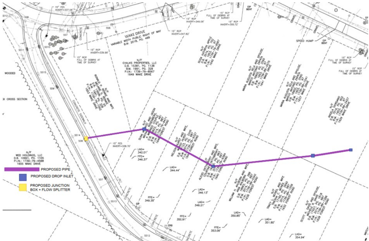
Figure 3: Alternative Pipe Alignment
