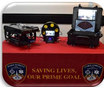
Members of the WFFD are currently being trained on how to maneuver the ROV and operate its computer system and controllers. Equipped with sophisticated sonar and navigation, the ROV can operate in dark murky waters in depths up to 1,000 feet.
